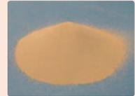
Newly-developed lead-free piezoelectric material
