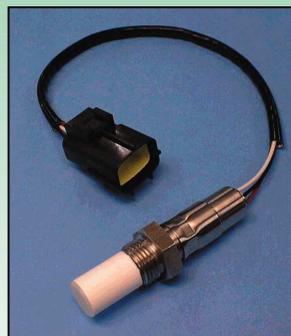
of their kind that can be installed on-board. For achieving practical application of fuel-cell vehicles, which automotive manufacturers are competing fiercely to develop, efficient control of hydrogen using these sensors will be indispensable. Besides application of these hydrogen sensors for fuel-cell vehicles, we intend to expand their application to stationary fuel cells for power sources, air-flow meters for gasoline or diesel engines, and other silicon micro-gas sensors.
