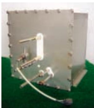
**A trial unit of 1kW SOFC power generation**
