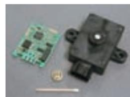
MEMS thermal conductivity type hydrogen sensors
